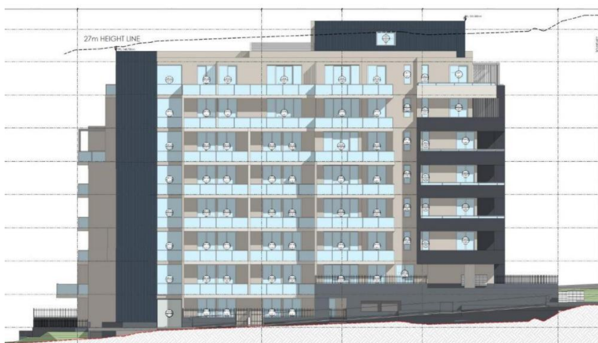
Figure 2: Southern (side) elevation showing the height breach
